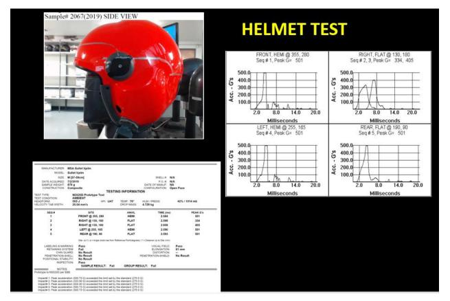
There was an MSA helmet failure during a GN Hydroplane crash at Cambridge, Maryland, USA during the 2019 season. The Gentex flight helmet is of similar construction. The allowable transmission of g loadings transmitted to the head form was considered proprietary by the company, however, the assumption can be made by examining the construction that this helmet is not intended for motor racing use.
