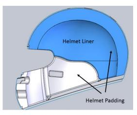
The padding inside the liner and between portions of the shell and the face may consist of a variety of closed cell foams often covered with nylon or a soft felt. Nomex fabric is often used in helmets that may be used in environments where the helmet might be exposed to fire.
