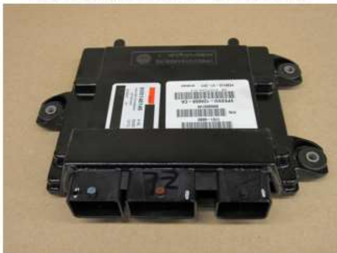
Engine control unit (ECU) – connector side
