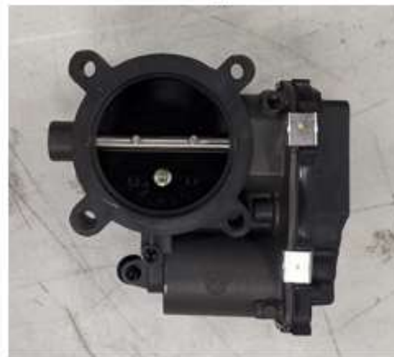
Throttle body – outlet side
