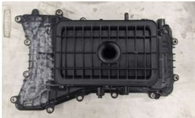
Port intake runners - inside
