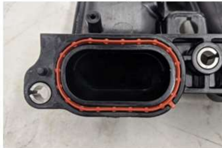
Throttle body – outlet side
