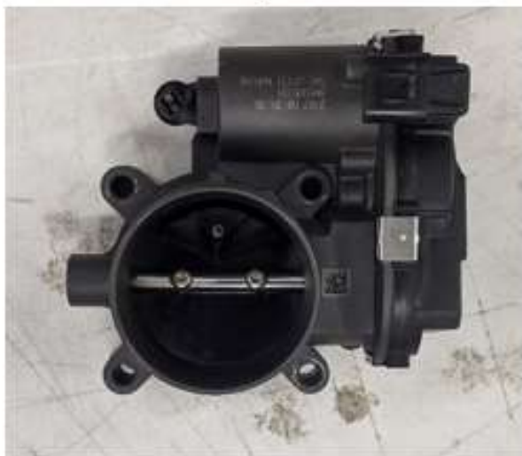
Throttle body – inlet side
