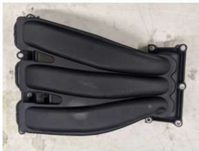
Starboard intake runners - outside
