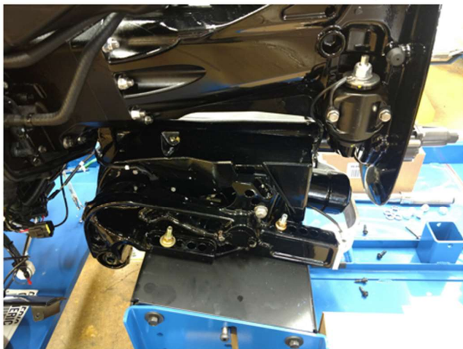
20" Transom bracket, 45° from the rear, port side
