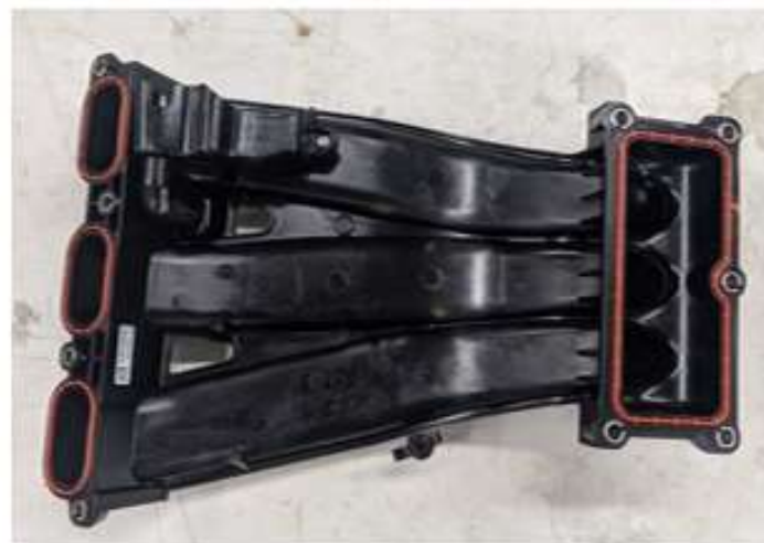
Port intake runners - inside
