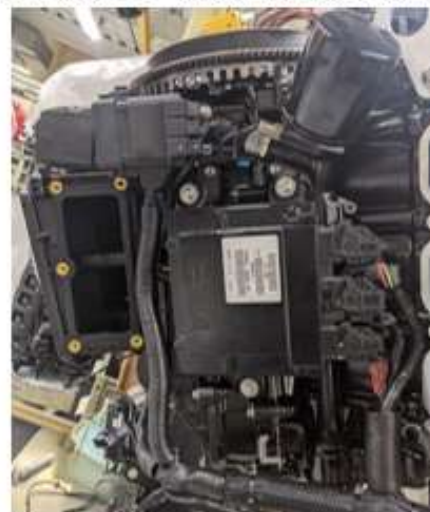
ECU on-engine – under port intake runners
