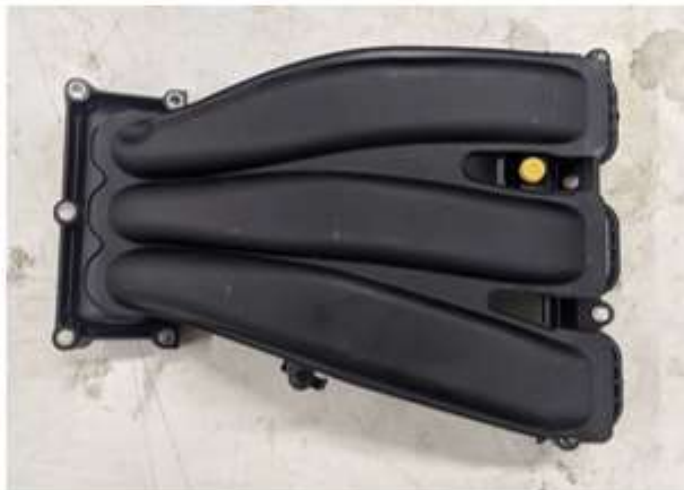
Starboard intake runners - outside
