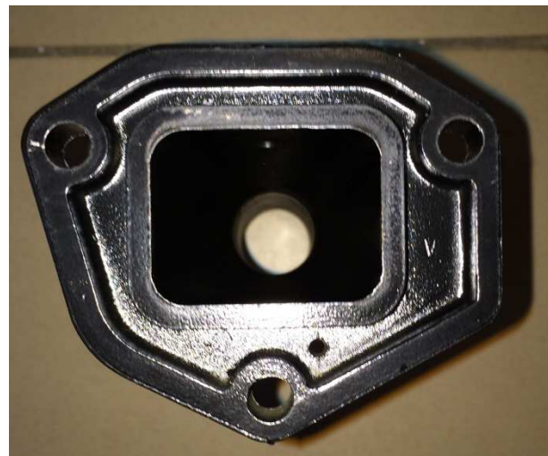
Internal exhaust tuner – viewed from engine side
