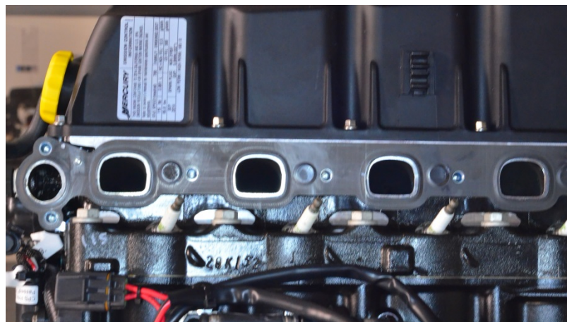
Cylinder head showing exhaust ports with gasket.
