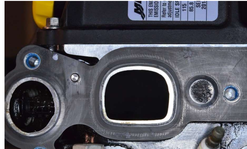
Cylinder head showing exhaust ports with gasket - detail
