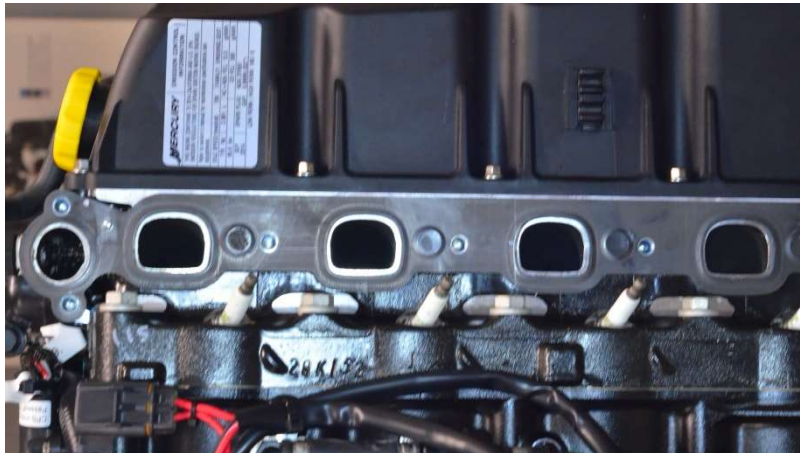
Cylinder head showing exhaust ports with gasket.
