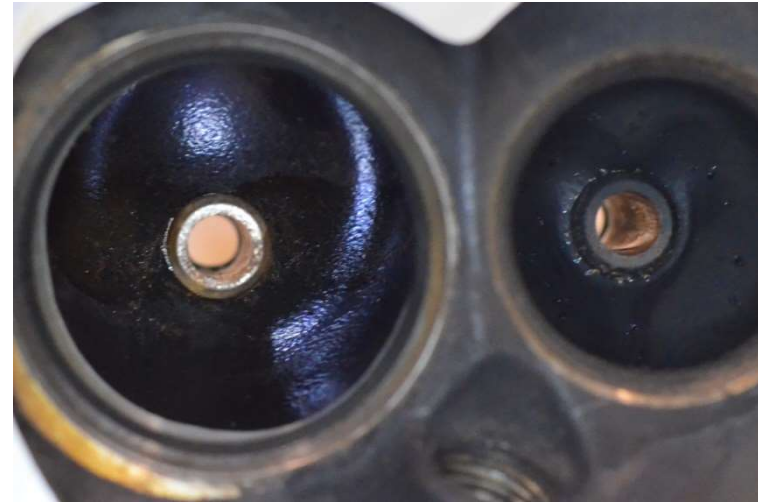
Cylinder head showing intake port
