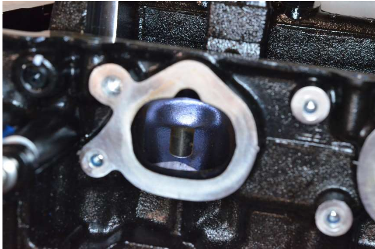
Cylinder head showing intake port.
