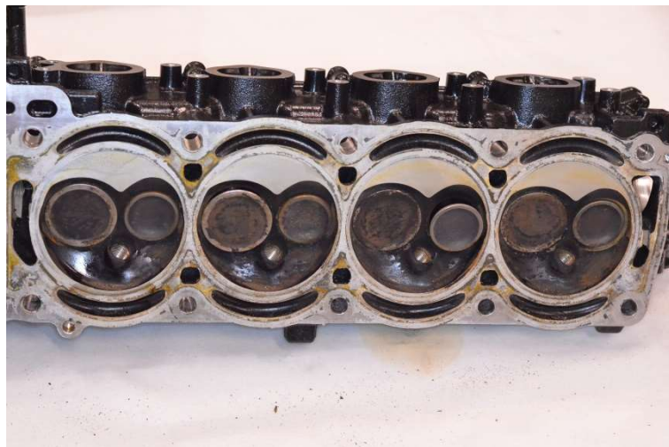
Cylinder head from the combustion chamber side
