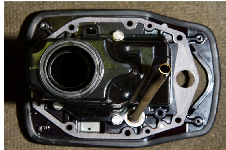
Internal exhaust tuner – viewed from gear case side
