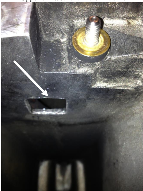
Upper exhaust relief hole in baffle
