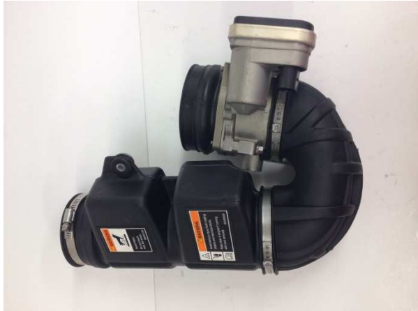
Intake silencer air intakes
