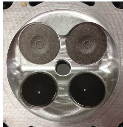
Combustion chamber – close up
