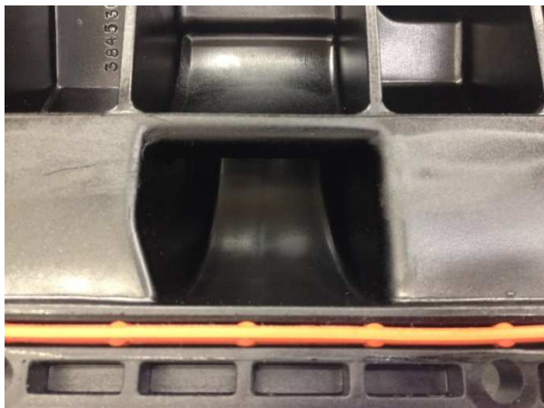
Intake manifold port - Close up – CAC side
