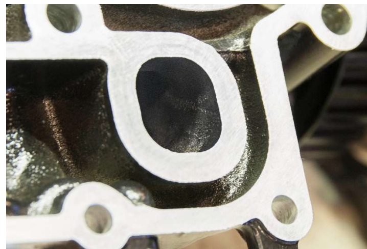
Cylinder head showing exhaust ports - detail
