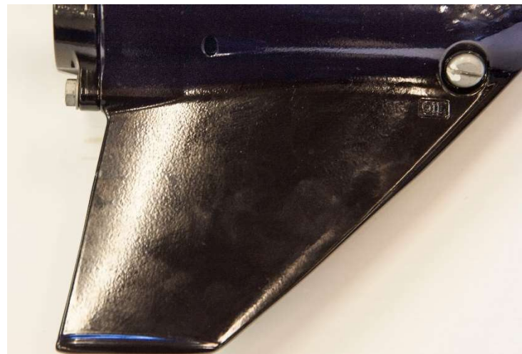
Gear house skeg - Close up from bottom side
