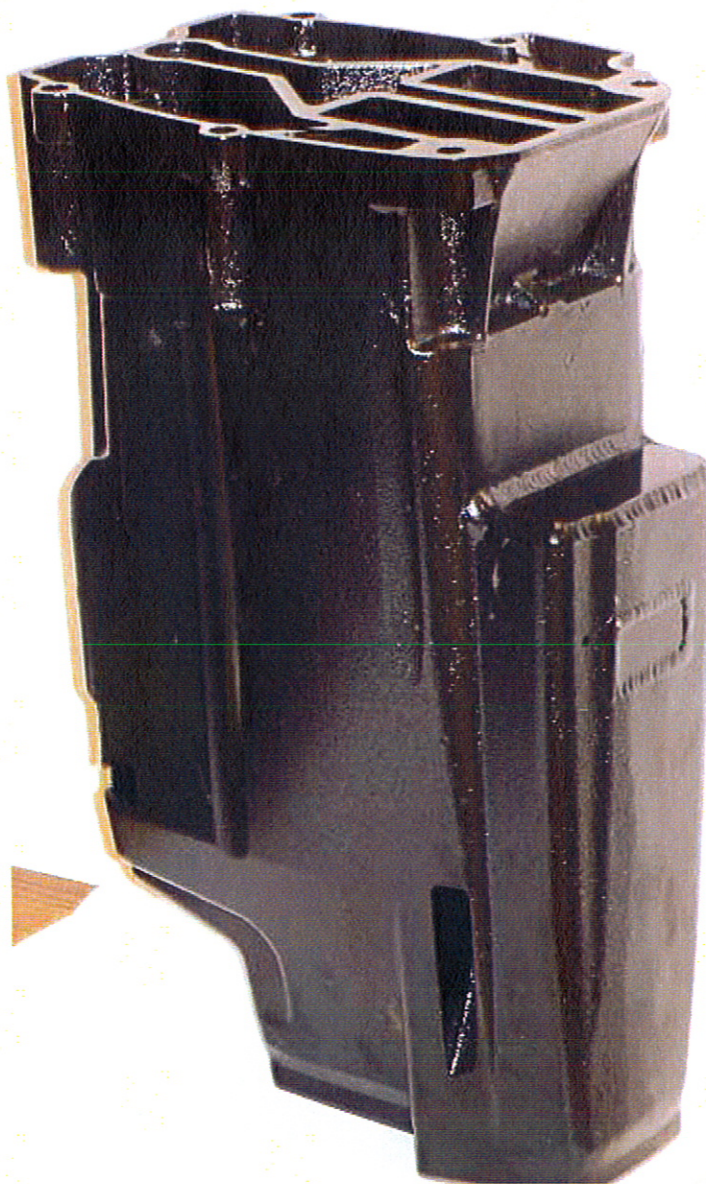
Exhaust tuner & muffler showing specific fabrication detail
