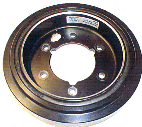
Harmonic balancer (fitted internally to flywheel)
