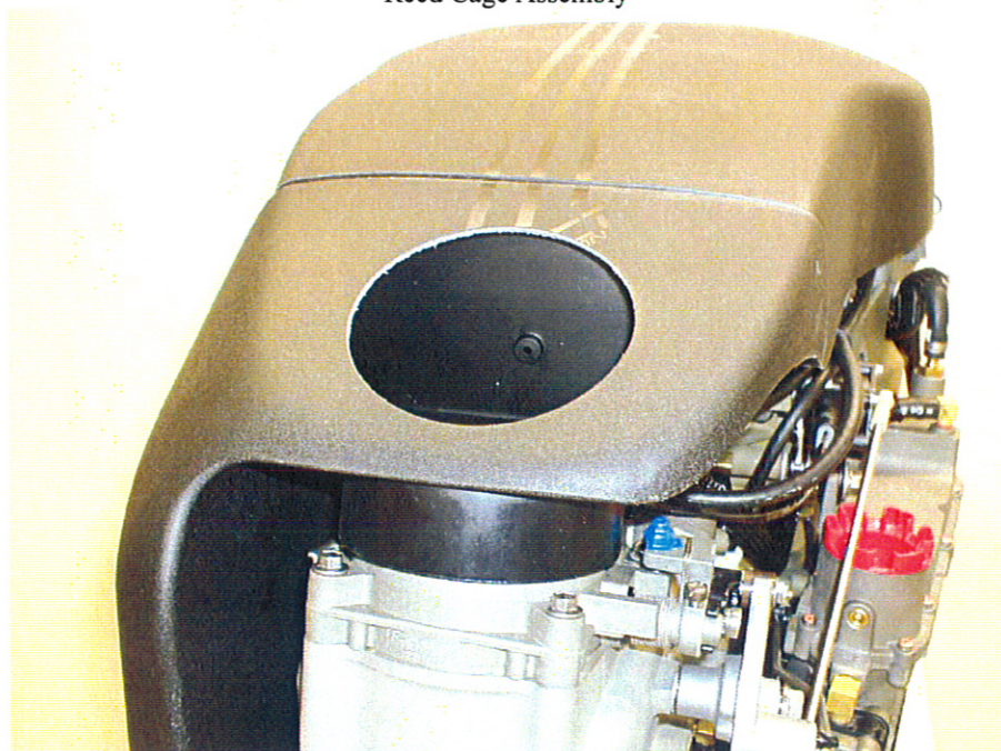
Sound Attenuator showing extra intake hole.
