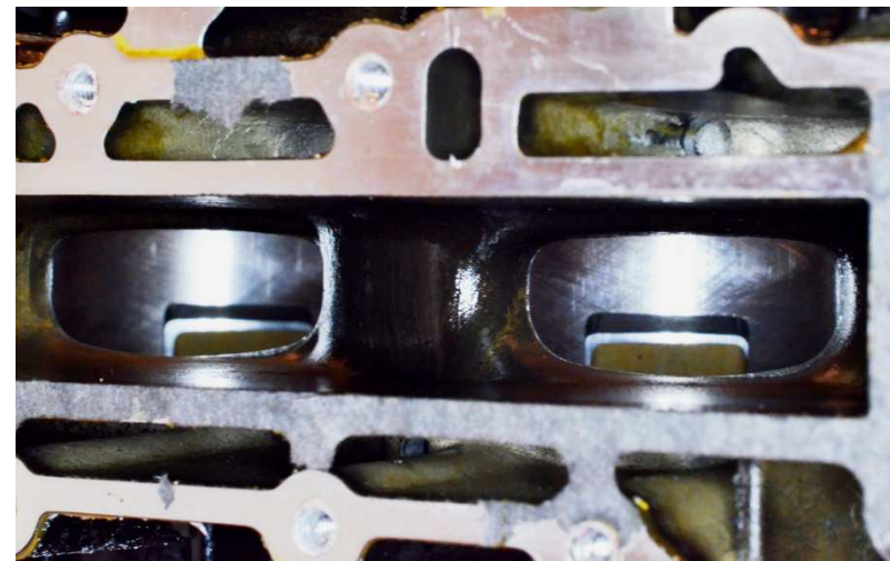
Cylinder block, showing exhaust port gallery
