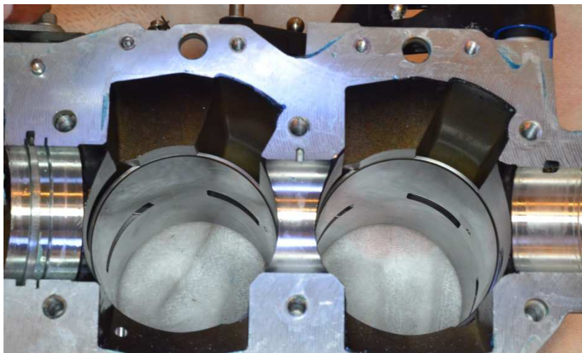
Cylinder block, viewed from crankshaft side.
