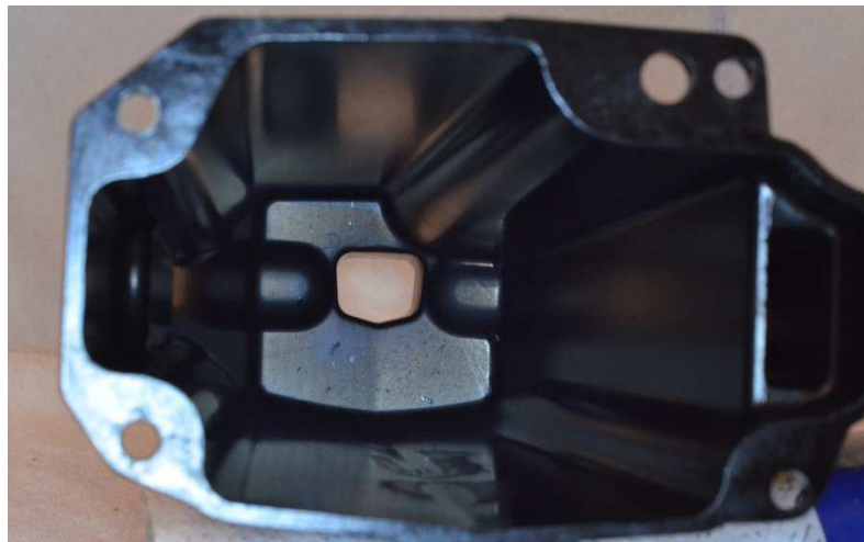
Internal exhaust tuner – viewed from gear house side
