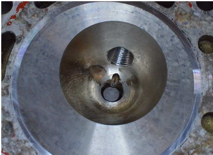
Cylinder head showing combustion chamber.
