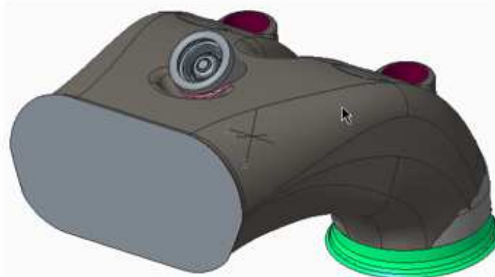
Intake port core from manifold flange to intake valves, including valve stems; maximum volume = 152 cc
