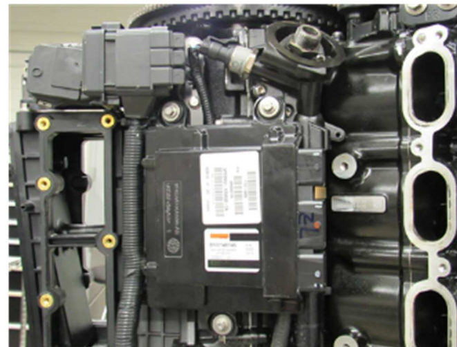
ECU on-engine – under port intake runners
