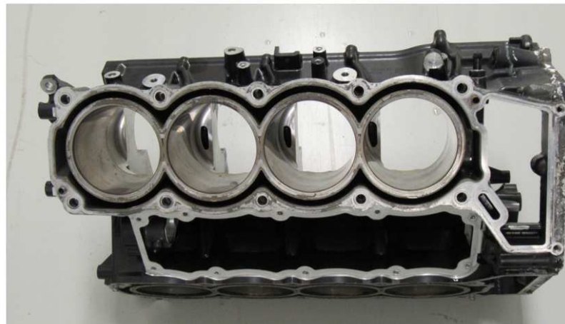
Cylinder block from crankshaft side
