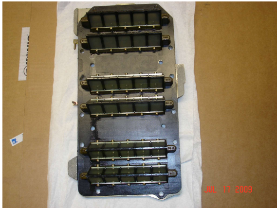
Crankcase half showing reed valve assembly
