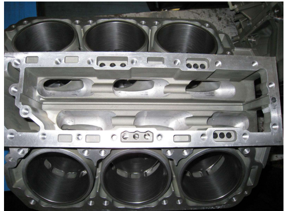
Cylinder block showing exhaust port gallery
