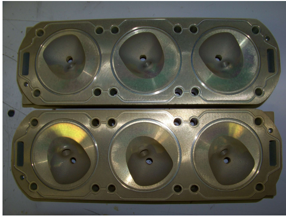
Cylinder head from the combustion chamber side
