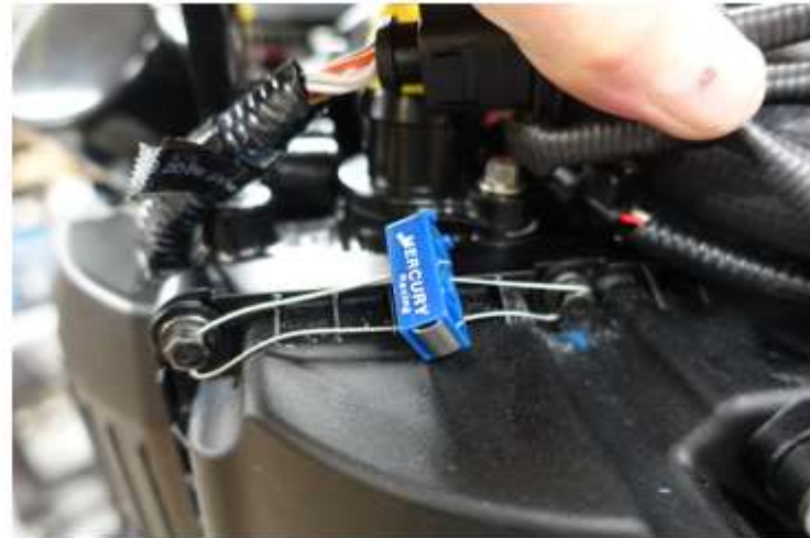
Anti-tamper device, port valve cover
