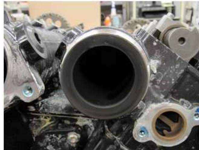
Intake port core from manifold flange to intake valves, including valve stems; maximum volume = 152 cc
