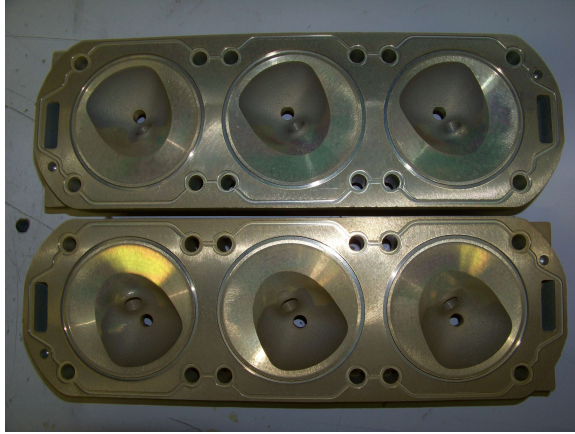
Cylinder head from the combustion chamber side
