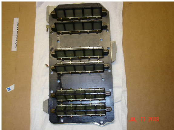
Crankcase half showing reed valve assembly
