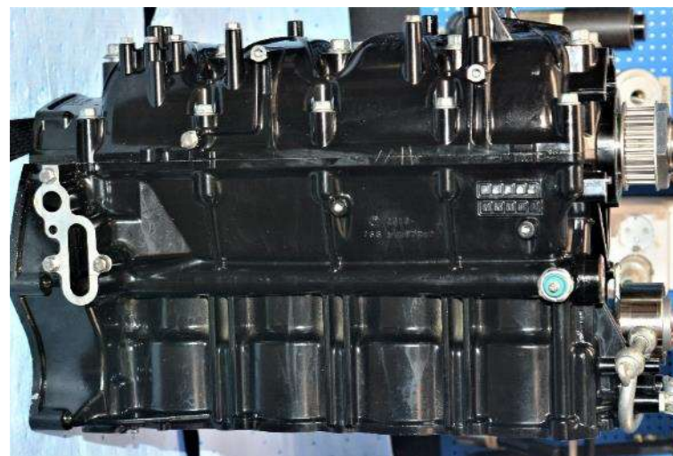
Cylinder block, port side
