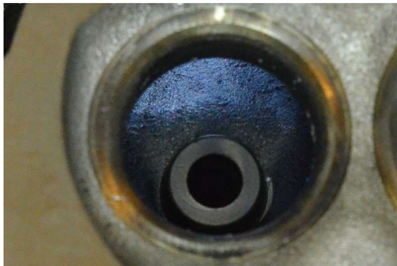
Cylinder head showing exhaust ports – from combustion side
