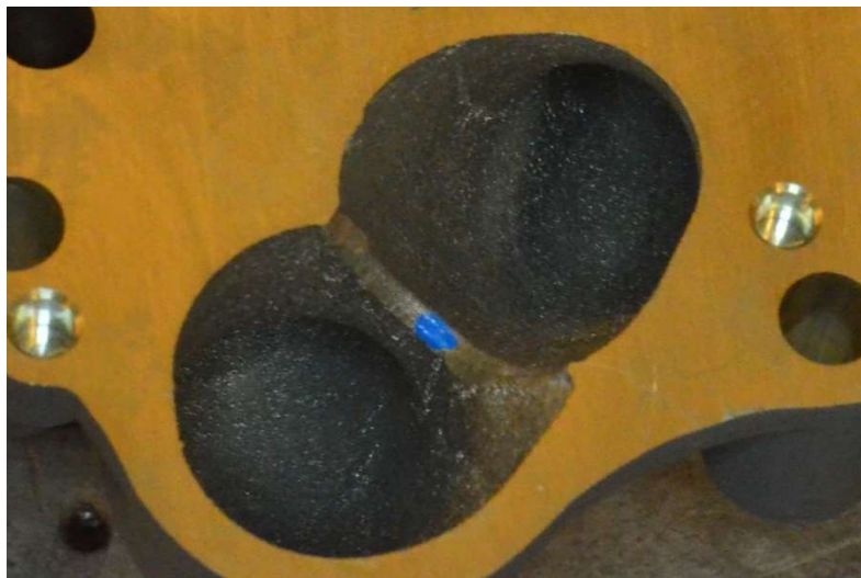
Cylinder head showing exhaust ports – from combustion side
