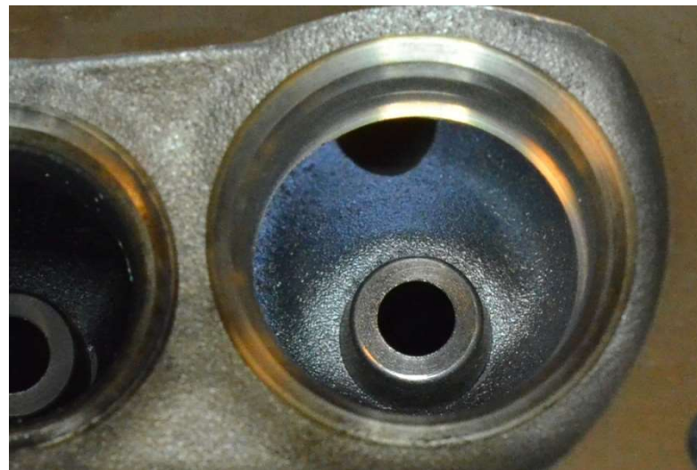
Cylinder head showing exhaust ports – from exhaust side
