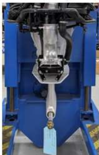
Midsection assembly and gearcase, aft side
