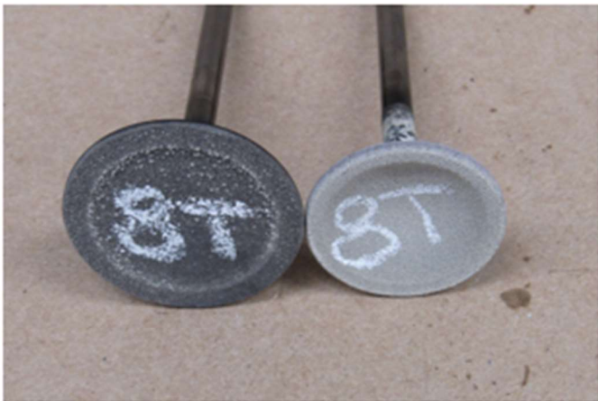
Intake (left) and exhaust (right) valves
