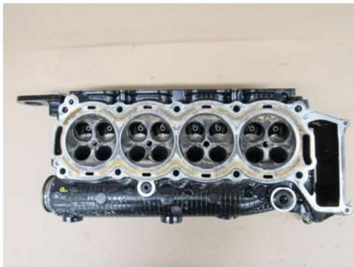
Cylinder head (port) from combustion chamber side
