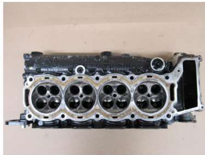
Cylinder head (starboard) from combustion chamber side
