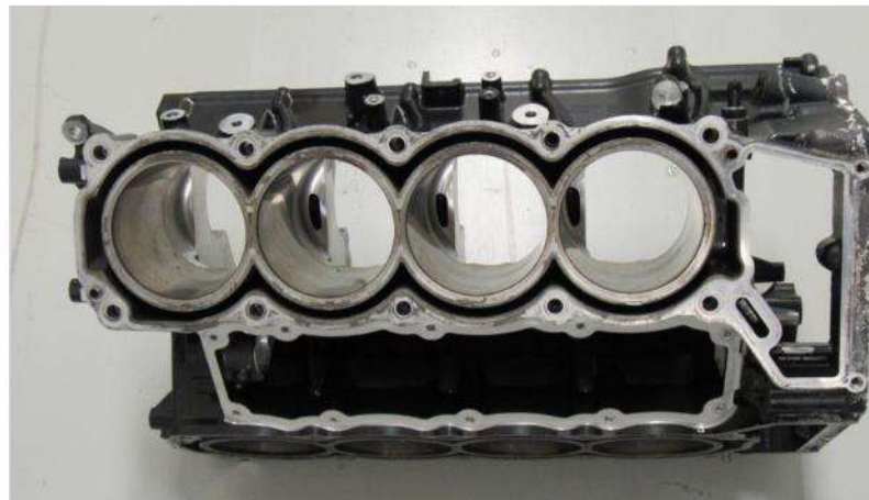
Cylinder block from crankshaft side
