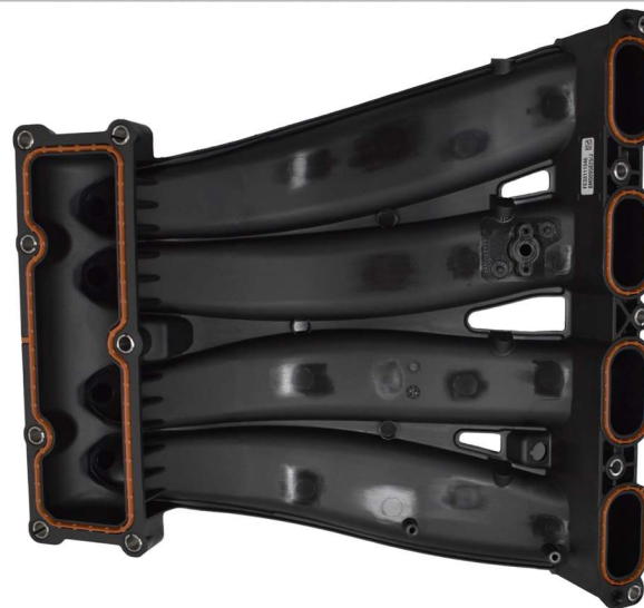
Intake manifold throttle adapter
