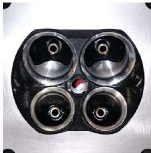
Combustion chamber without valves
