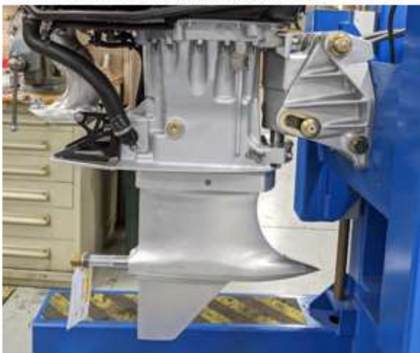
Midsection assembly and gearcase, stbd side
