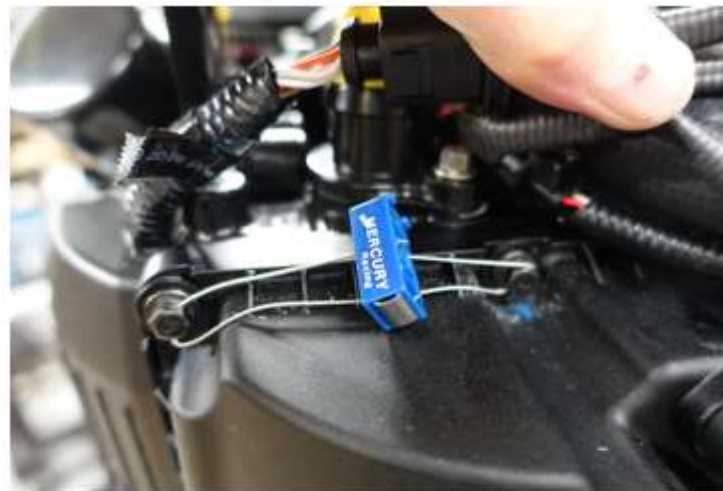
Anti-tamper device, port valve cover
