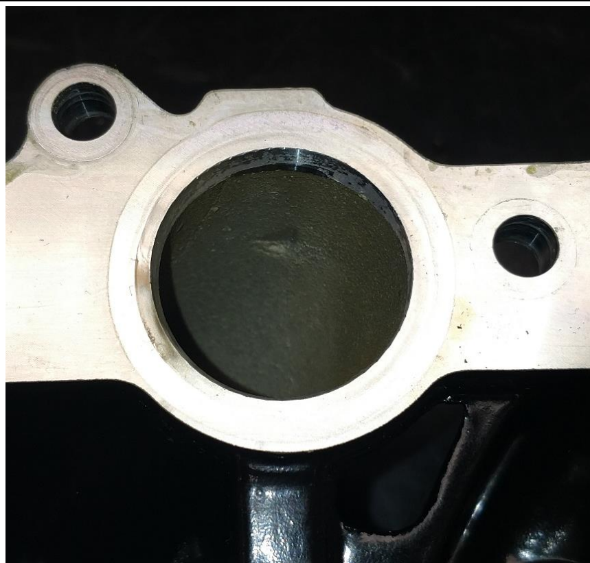
Cylinder head showing intake ports.
