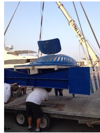
Dunk test cockpit and frame. Cockpit rotates within the frame.
