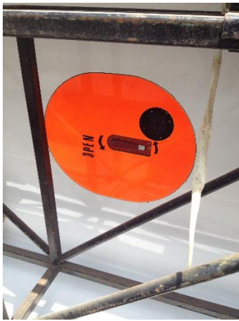
Escape hatch in tunnel of XCAT hull.
